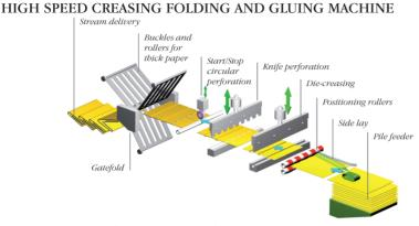
The Cordoba range follows the rule of using a matrix system to crease substrates prior to folding. Heavy boards or plastics, or laminations in addition to cross grain or digitally printed works can now be created without a die-cutting machine.
