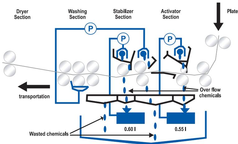
The SDP-Eco1630IIR features a self-contained Eco processor that operates with two, ready-to-use solutions for processing Silver DigiPlate. This unique processing technology uses 2/3 less Activator and Stabilizer than other systems.
